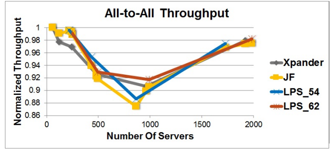
(b) k = 18 . There are 4 servers placed under each switch.
